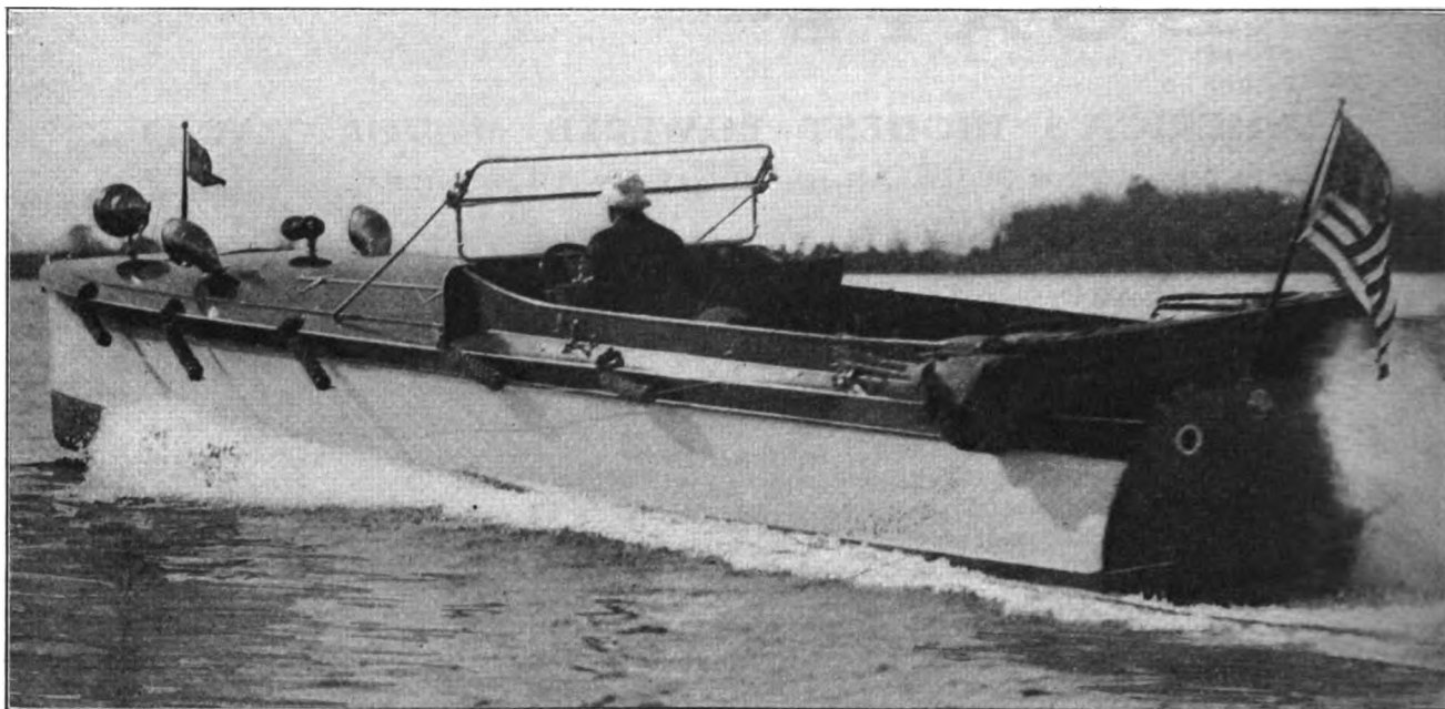
A Thirty-Five-Foot Ramaley Runabout as Owned by Senator D. F. Harding, Jr., of Chicago. She is Powered with Six-Cylinder 100-H.P. Van Blerck Equipped with a Leece-Neville Electric Starter. Speed 32 Miles per Hour
